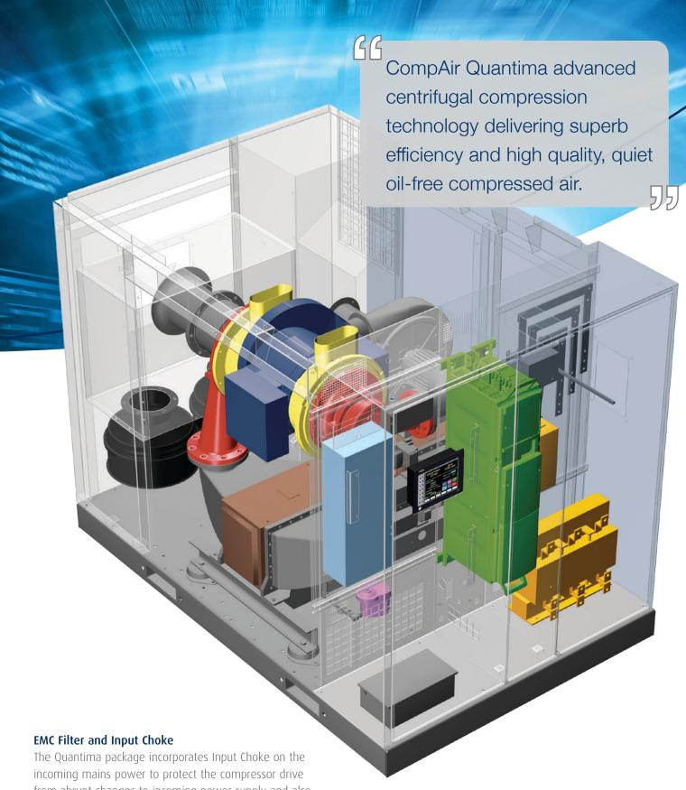
The Quantima package incorporates Input Choke on the incoming mains power to protect the compressor drive from abrupt changes to incoming power supply and also function as protection against harmonics back to the mains supply. An EMC filter is also fitted to attenuate any electromagnetic noise at higher frequencies that may cause harm to external equipment.
